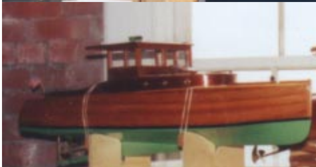
(Lower Left) 1920s Cabin Cruiser Radio Control 36-Inch Model (#60, Case 1). Design: Classic Raised-Deck Cruiser. Scratch-Built 2001 Using Planked-on-Frame Hull. Builder/Owner: Al Hubbard.
