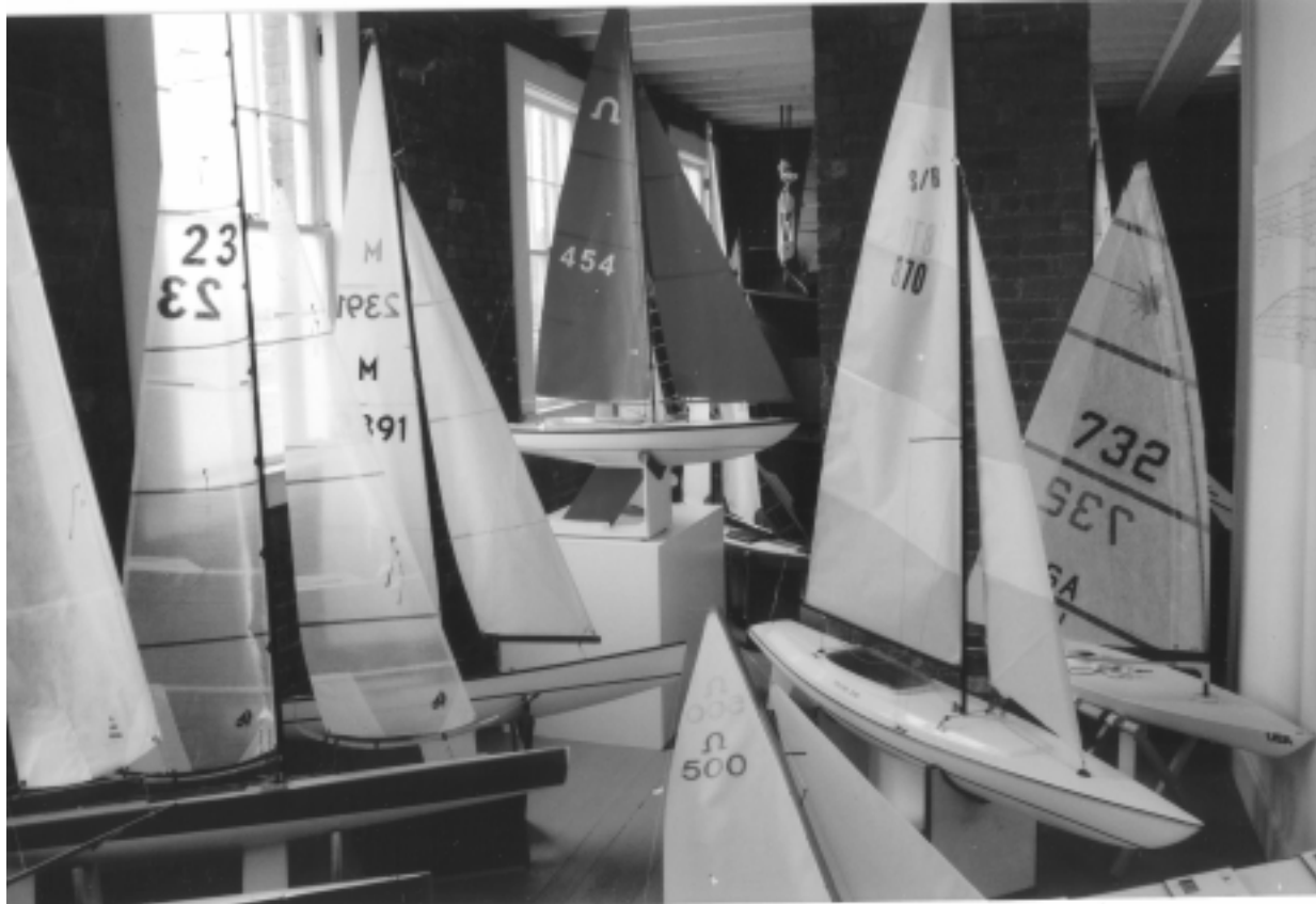
Sail Number 23: 1990s Skinny M Class Radio Control 50-Inch Yacht (#36, Zone 6). Swede Johnson M Design with Stayless Swing Rig. Scratch-Built 2002 with Johnson Fiberglass Hull. Builder/Owner: Ben Martin; 391: 1980s Archer M Class Radio Control 50-Inch Yacht (#35, Zone 6). Jon Elmaleh M Design with Conventional Sail Rig. Scratch-Built from Elmaleh Carbon Fiber Hull. Owner: Greg Vasileff; 454: 1973 Larita Soling 50 Class Radio Control Yacht (#33, Zone 6). John & Laurie Converse One-Design from Full-Scale Soling . Scratch-Built from Vortex Model Engineering Fiberglass Hull. Owner: Art Hart; 870:1973 Tricks End Santa Barbara Class Radio Control 70-Inch Yacht (#37, Zone 6). Tom Protheroe One-Design Based on 1960s Era Yacht Designs. Scratch-Built with Protheroe Fiberglass Hull/Deck; Military Drone Winch. Builder/Owner: John Garbarino; 732: 1995 RC Laser Class Radio Control 42-Inch Yacht (#32, Zone 6). One-Design by Bruce Kirby and Jon Elmaleh from Full-Size Laser Yacht. Out There Technologies LLC Polyethylene Kit. Owner: June Pendino
