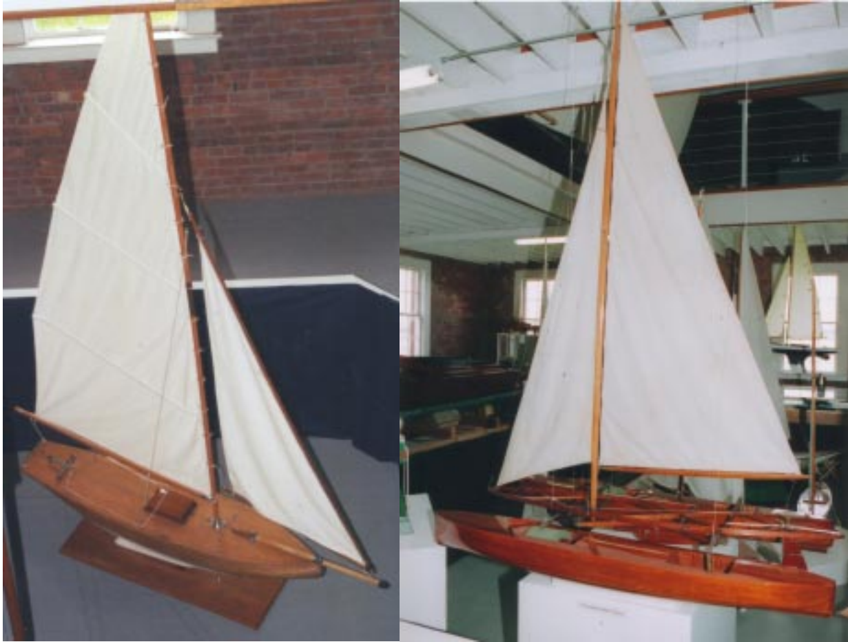
(Left) 1930s (Est.) "Christchurch Four Foot Six" NZ Class Free Sailing 54-Inch Yacht (#19, Zone 7). New Zealand Design with Full-Battened Mainsail and Braine Steering. Scratch-Built with Planked Hull from Native NZ Wood. Restored by Christchurch MYC Members in 2004. Owner: Min Sarginson
