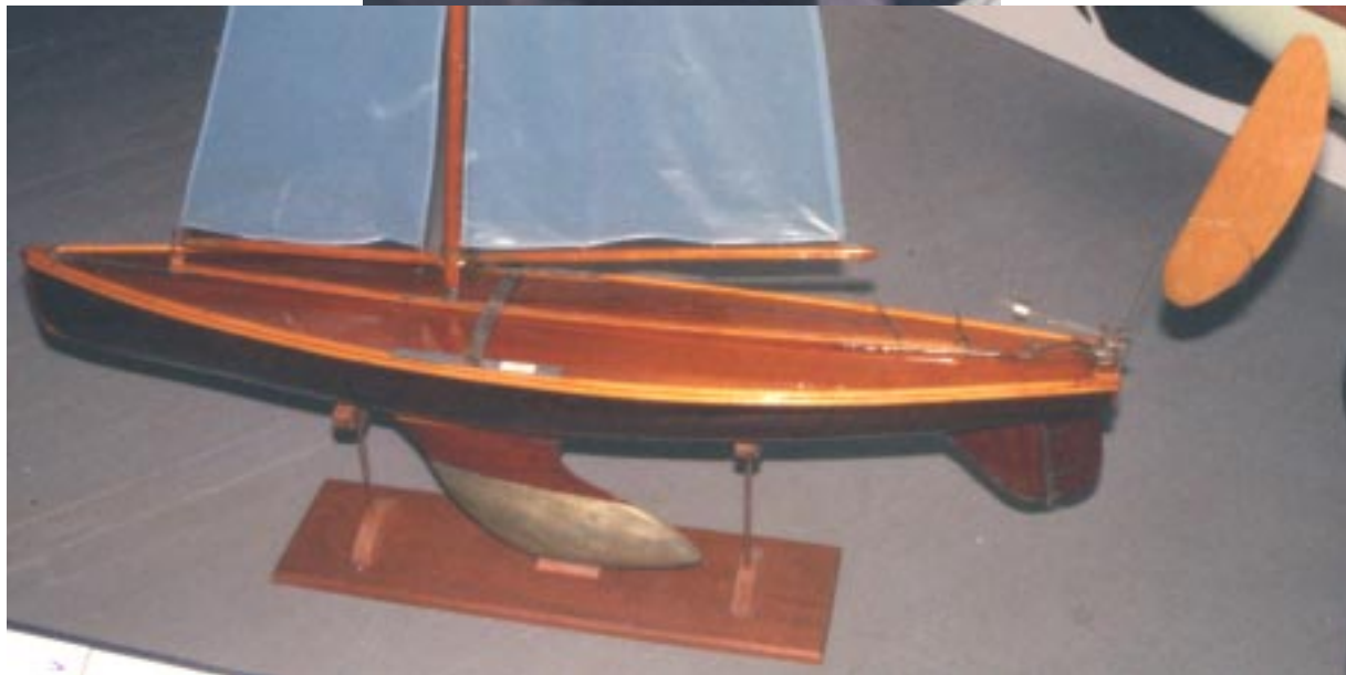
1936 Cheerio I M Class Olympic Radio-Control Radio Control Yacht (#E-1, Entryway) . John Black Design. Scratch-Built 2000 from Fiberglass Hull. Builder/Owner: Art Hart
