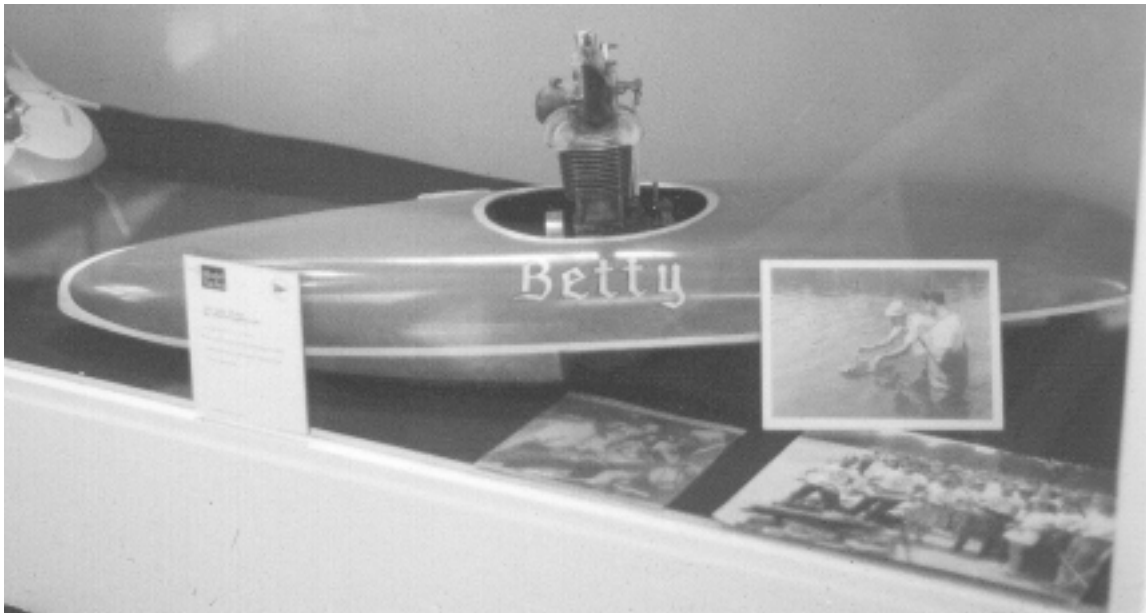
1937 Betty 36-Inch Gas Tetherline Speedboat (#51, Case 1). George Tanner, N.A., Designer; Bob Adams, Detroit Builder; Solid Sugar Pine Block. Homemade Motor with Unique Outdrive Design. Owner: Kent Lund
