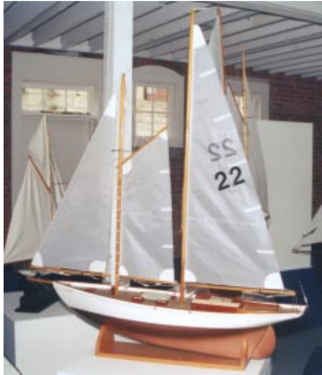
(Top Left) 1905 Elizabeth Silsbee Radio Control 93-Inch Topsail Fishing Schooner (#2, Zone 1). W. Starling Burgess Traditional Full-Scale Design. Scratch-Built 2000 with West Epoxy/Fiberglass Cloth Hull. Builder/Owner: Andrew Charters
