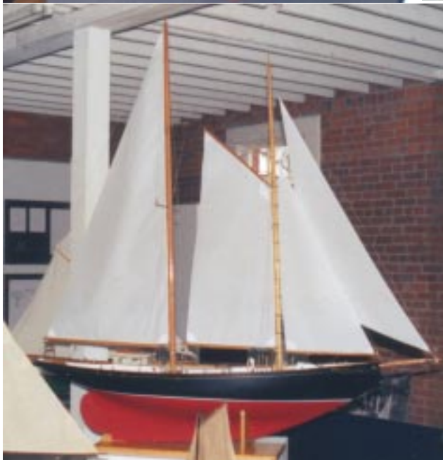
(Top Left) 1905 Elizabeth Silsbee Radio Control 93-Inch Topsail Fishing Schooner (#2, Zone 1). W. Starling Burgess Traditional Full-Scale Design. Scratch-Built 2000 with West Epoxy/Fiberglass Cloth Hull. Builder/Owner: Andrew Charters
